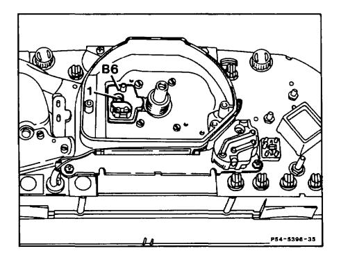
Securing screw (1) ...... remove, insert. Hall sensor (B6) ..... take off, insert.
