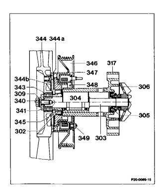
The armature (344a) is attracted by the magnet body (347) and presses against the face of the belt pulley (346).
