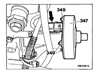
The belt pulley (346) is fitted on the coolant pump shaft ahead of the magnet body.
