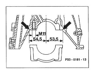
The forged conrods are guided axially in the pistons (piston-guided conrods) (arrows).
