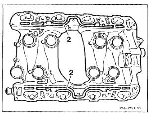
The quantity of fuel vapours and blow-by gases allocated to the individual cylinders is metered through restriction openings (3) in the intake manifold gaskets.
