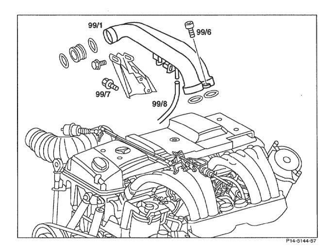
Bolt (99/6) at resonance intake manifold ..... unscrew, screw in.
