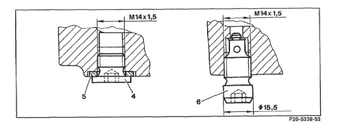
Drain plug (6) (2nd version) with fitting taper for drain hose and captive seal must not be used on the crankcase with drain plug (4) (1st version).
