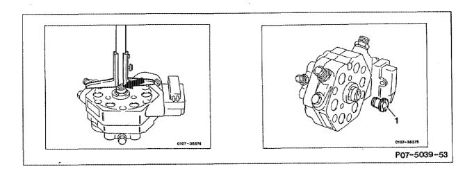
Position (arrow) of screw plug measure with depth gauge and note. Mark position with marking tool as a safeguard.
