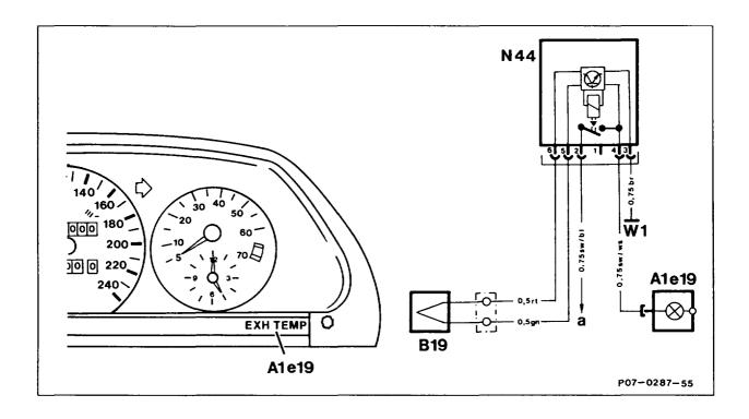
A1e19 Catalytic converter overheating warning lamp
